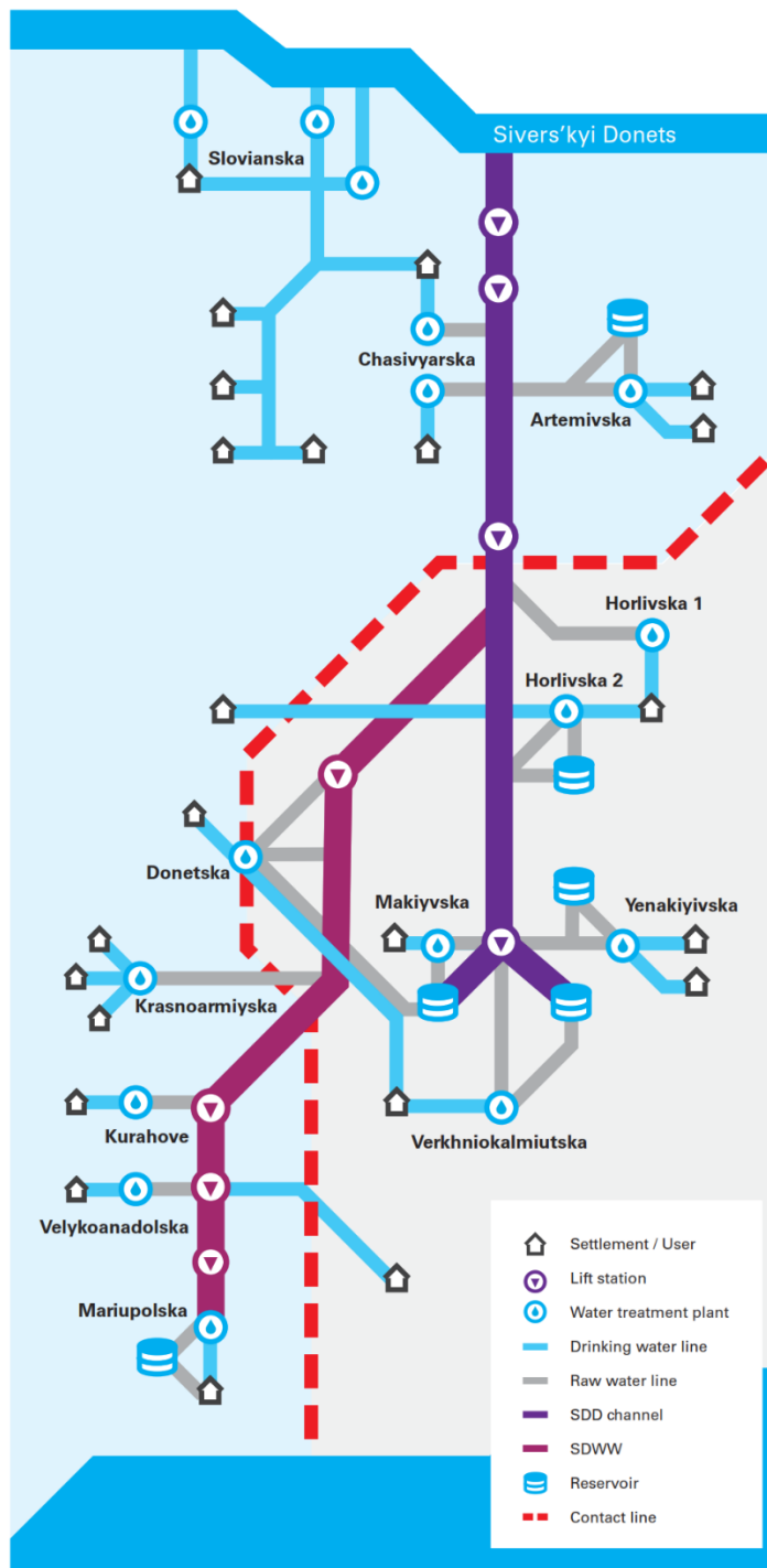
Simplified scheme of water supply system operated by Voda Donbasu company (source: UNICEF, Risk assessment of the "Voda Donbasu" water system Report, 2019)
